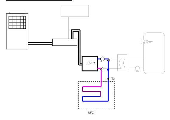
If UFC is required, it is almost inevitable that UFH will also be utilised. Therefore, UFC always requires an ACH1 and PAR21 to enable changeover between modes/set points.
