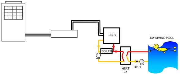
If the PQFY was installed on a swimming pool which had heavy and constant use with large heat losses, a top up boiler in parallel can be used. The PQFY can maintain the temperature of the pool at around 30°C, however over time this temperature may slowly drop. When, for example, the temperature reaches 28°C, the boiler comes on and heats the pool back up to 31°C. The PQFY may heat the pool for several days before the temperature drops by 1°C.
