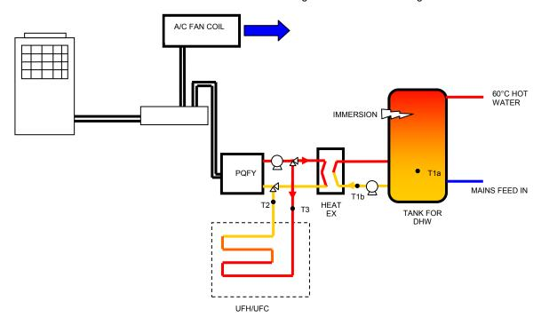
Below is an explanation of each PQFY configuration with the addition of fan coils/units to the system.
