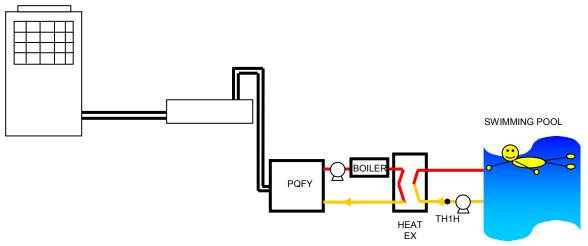
If an existing boiler is being used, a PQFY can be used to supplement the heat load, to take load off the boiler. Also this set up can be used if the PQFY is required only to take part of the demand from the boiler.
