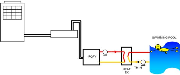
This is the case when the heating system for a swimming pool is being covered completely by the PQFY, for example on new build or new heating install.
